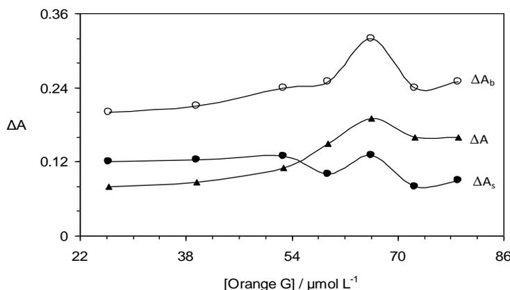
**Fig. 2:** Effect of Orange G concentration on the rate of uninhibited ( $\Delta A_b$ ), inhibited ( $\Delta A_s$ ) reactions and response ( $\Delta A$ ). (Conditions: sulfuric acid,  $0.4 \text{ mol L}^{-1}$ ; codeine,  $25.0 \text{ } \mu\text{mol L}^{-1}$ ; bromate,  $2.5 \text{ mmol L}^{-1}$ ;  $25 \text{ }^\circ\text{C}$  and  $450 \text{ s}$ ).
