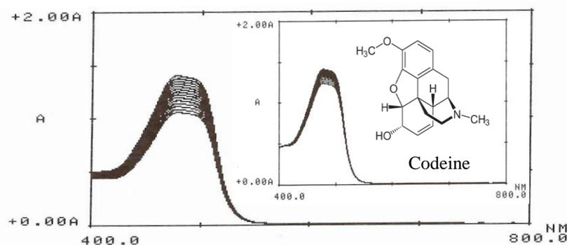
**Fig. 1: Absorption spectra of the uninhibited reaction. (Conditions: Orange G, 1.2 mL of  $6.6 \times 10^{-4}$  mol L<sup>-1</sup>; sulfuric acid, 1.0 mL of 4.0 mol L<sup>-1</sup>; bromate, 0.5 mL of 0.05 mol L<sup>-1</sup>; 25 °C and 7.5 min). Inset shows the absorption spectra of the inhibited reaction in presence of 25.0 μmol L<sup>-1</sup> of codeine.**
