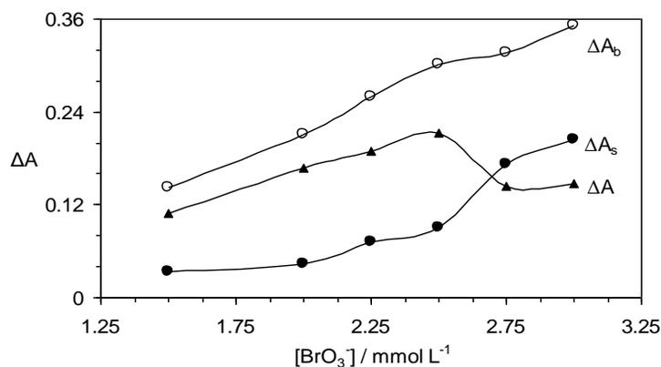
**Fig. 4:** Effect of bromate concentration on the rate of uninhibited ( $\Delta A_b$ ), inhibited ( $\Delta A_s$ ) reaction and response ( $\Delta A$ ). (Conditions: Orange G,  $66.0 \mu\text{mol L}^{-1}$ ; sulfuric acid,  $0.44 \text{ mol L}^{-1}$ ; codeine,  $25.0 \mu\text{mol L}^{-1}$ ;  $25^\circ\text{C}$  and  $450 \text{ s}$ ).
